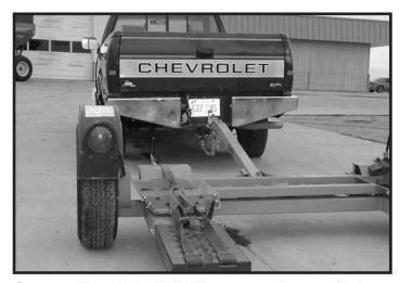
Step 13. To pull the TOW-IT empty, make sure tie-down straps are tightened in the storage position, and towed vehicle safety chains are wrapped up and hooked. Tie-down winch handles should be left in a down position (horizontal) with safety pins in place when towing loaded or empty. DO NOT ATTEMPT TO PULL TOW-IT WITH WHEEL PLATFORM IN LOADING (tilted) POSITION.
